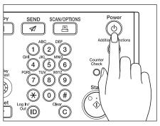
To turn the control panel ON or OFF, press the control panel power switch. When the control panel is turned OFF, the machine is in the Sleep mode.
